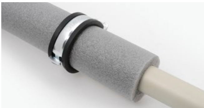
In the case of hot water, sleeve is installed with insulation that is larger by one dimension.
